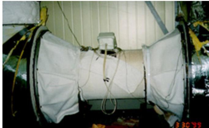
HIGH TEMPERATURE FAN TESTING Max. Dia. 2,060 mm Max. Length 1,200 mm Max. Temp. 400 °C
